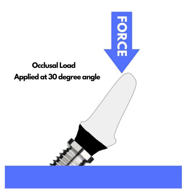
They found that the arrangements with two implants actually had a higher fracture resistance value than the ones with one implant. So, adding an extra implant can help strengthen the entire thing!
